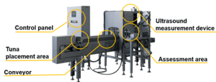
Figure 1. Diagram of the SONOFAI T-01
